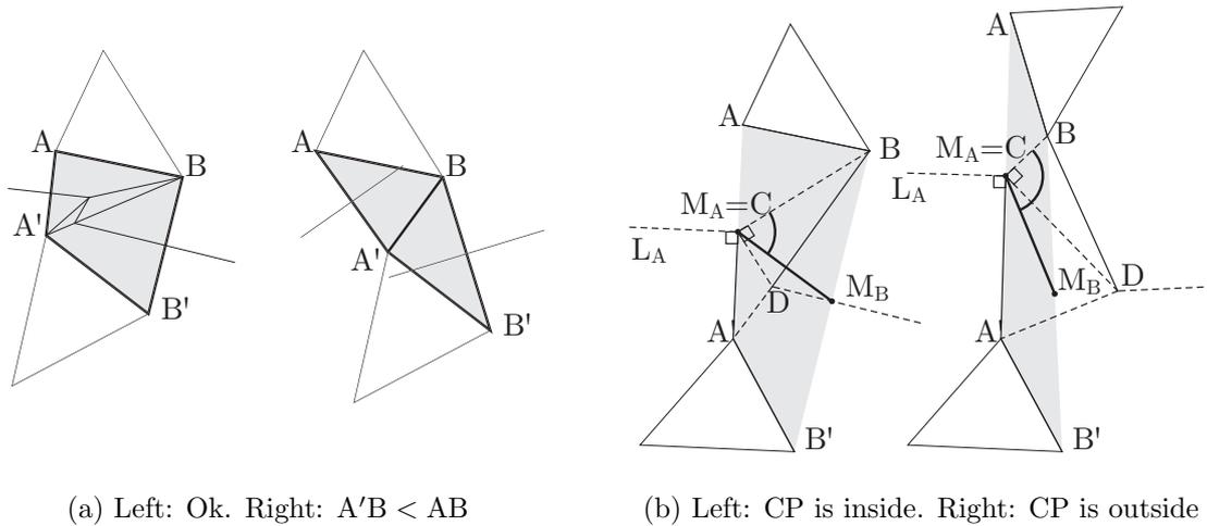
Figure 6: Conditions for an edge-tucking molecule. (a) Conditions to generate crease pattern. (b) Conditions for making the crease pattern inside the molecule.
