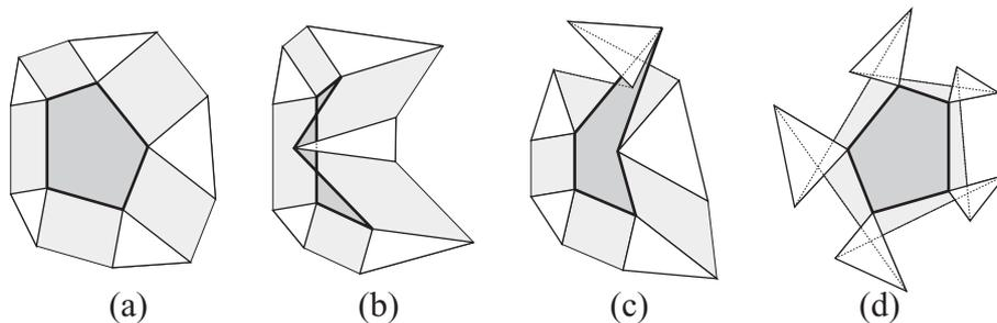
Figure 4: Conditions for properly tessellation. (a) Ok. (b) The vertex-tucking molecule is crossed. (c) The edge-tucking molecule is crossed. (d) The vertex-tucking molecules and edge-tucking molecules have negative area.
