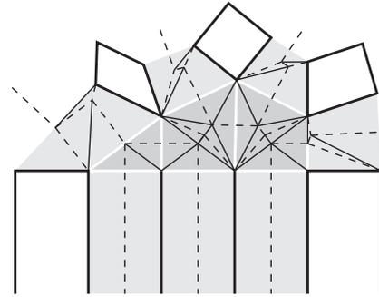
(b) Connecting 3D design (top) to regular box pleating pattern (bottom).
