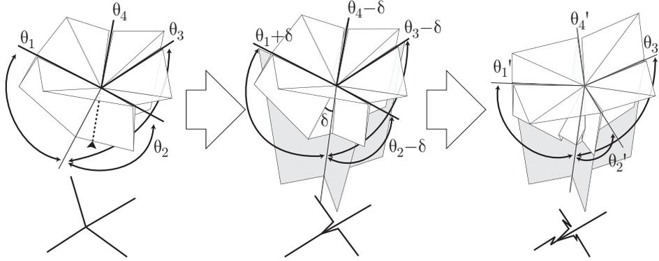
Figure 11: Adjusting tuck angles. (Left to Middle) One of the tuck angles is increased by moving the joint axis. (Middle to Right) Any tuck angles can be reduced by crimping.
