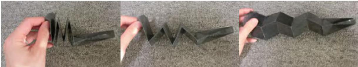
Figure 10: Capped tube theoretically, infinitesimally flexible at  $75^\circ$  and stable at  $45^\circ$ .
