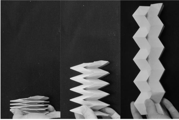
**Figure 10:** A glide-reflection coupling of tubes [22] actuated from one end. The stiffness of the 8th mode helps to achieve the uniform, steady deployment
