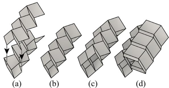
**Figure 9:** (a) Miura-ori sheets, (b) origami tube [23], (c) parallel alignment [23], and (d) glide-reflection coupling [22]
