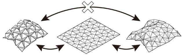
**Figure 17:** A mistake in the folding (right) can be fixed (left) only through returning to the entirely unfolded state (middle)
