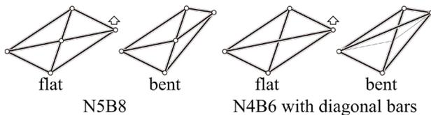
**Figure 8:** The N5B8 with hinge stiffness can model consistent bending stiffness. The N4B6 model with diagonal bars can be extremely stiff in its bent state as it forms a tetrahedron
