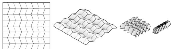
**Figure 12:** Miura-ori is an overconstrained mechanism
