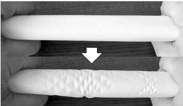
**Figure 3:** Buckling patterns of thin sheets are characterized by sharp creases
