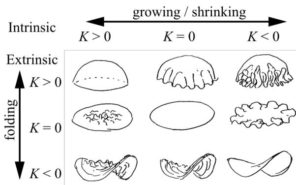
**Figure 7:** 3D to 3D folding allows for isolation of the intrinsic and extrinsic curvatures. Vertical direction corresponds to folding, while horizontal direction requires growing or shrinking of the material. This contrasts with a smooth ( $C^2$ ) surface along the diagonals, where intrinsic metric and extrinsic curvature correspond
