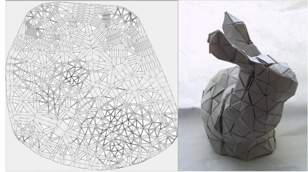
**Figure 4:** Crease pattern (left) computed by Origamizer and the folded model (right)
