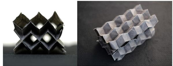
Figure 15: Interleaved tubular structure [38].
