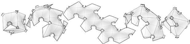
**Figure 19:** A structure that folds into a cube and an octahedron [46]
