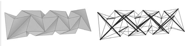
Figure 14: Shaky polyhedron (left) and tensegrity structure (right)
