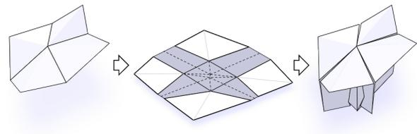
**Figure 5:** Folding up to close the gap using a crease pattern based on the Voronoi diagram
