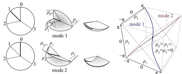
**Figure 18:** The configuration space of a degree-4 vertex (right) and its corresponding folding modes (left)
