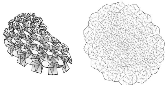
**Figure 6:** Freeform origami tessellations by generating Resch-type tessellations on a given surface. Computed using Freeform Origami
