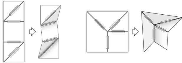
**Figure 11:** Left: serial linkage origami without a loop. We can assign arbitrary fold angles to all creases. Right: parallel linkage origami forming a loop around an interior vertex. The fold angles are geometrically constrained
