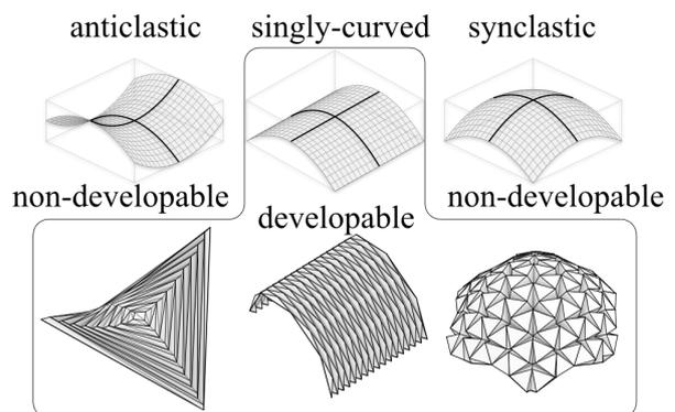
**Figure 2:** Top: smooth developable surfaces can form only singly curved surfaces. Bottom: creased surfaces allow for doubly-curved developables (pleated hyperboloid, Yoshimura-pattern, Resch's pattern)
