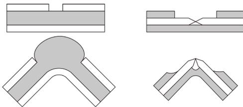
**Figure 16:** Swelling the middle layer[41](left) or shrinking the outer layer[42](right) leads to self-folding
